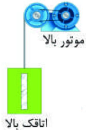
$$\bar{P} = \frac{W}{t} = \frac{mg\Delta h}{t} = \frac{500 \times 9.8 \times 4}{1} = 2940 \text{ W}$$
